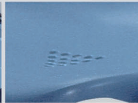
◆ Ventilation and Drain hole
